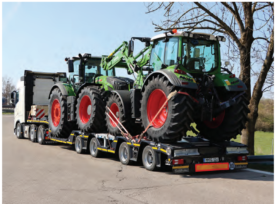
TOP AND ABOVE: The newly upgraded Stepstar semi lowloader from Goldhofer comes with a choice of one or two pairs of wheel recesses. This enables extremely high construction machines to be transported where maximum height regulations would otherwise be a problem.
