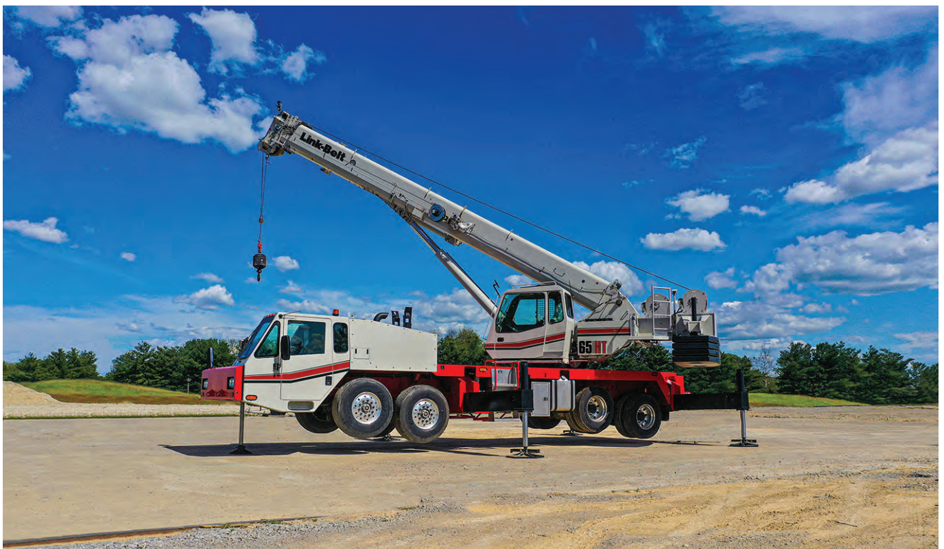
TOP AND ABOVE: The new 65|HT truck crane offers a 55 mt capacity. It is intended to replace Link-Belt's HTC-8660 Series II model.
