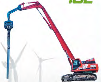
Excavator Vibro Hammer
