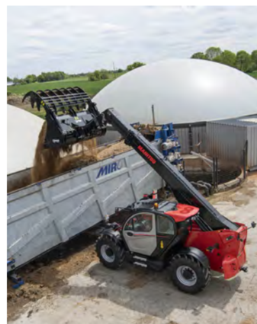
ALL IMAGES: The MLT 961-160 V+ L is currently the most powerful model in Manitou's NewAg XL range. The machine has a lifting capacity of up to 6 t for a lifting height of 9 m.
