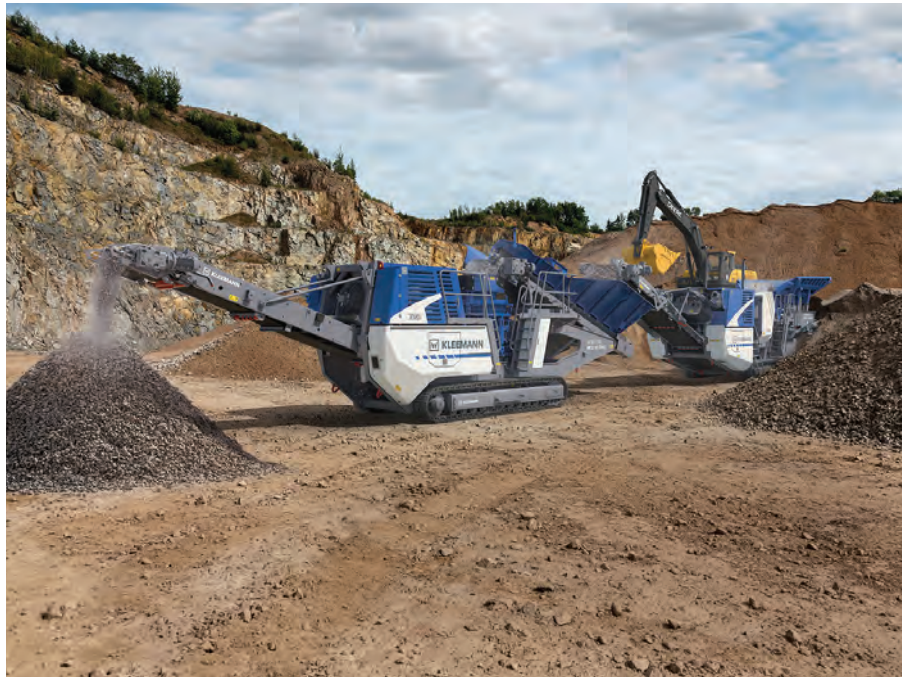
ABOVE: The new Mobicone MCO 90(i) EVO2 mobile cone crusher (on the left) has a feed capacity of up to 270 t/hr. The machine can be used together with the Mobicat MC 110(i) EVO2 mobile jaw crusher.
