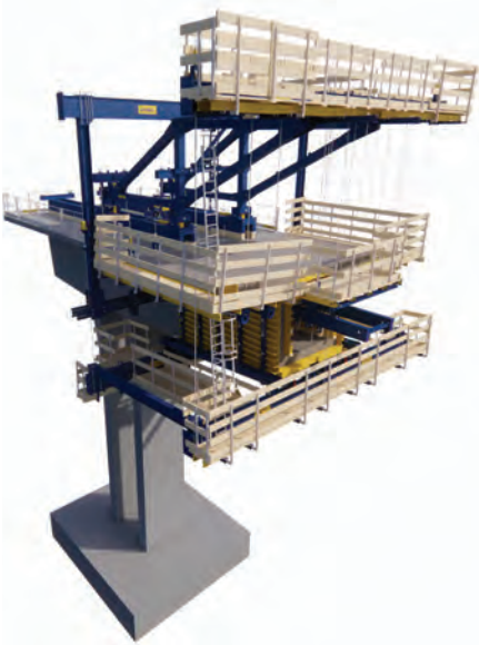
ABOVE, MIDDLE AND FAR RIGHT: The virtual formwork planning of the cantilever forming traveller (CFT) system using the DokaCAD for Revit software supported project implementation on the actual construction site.
