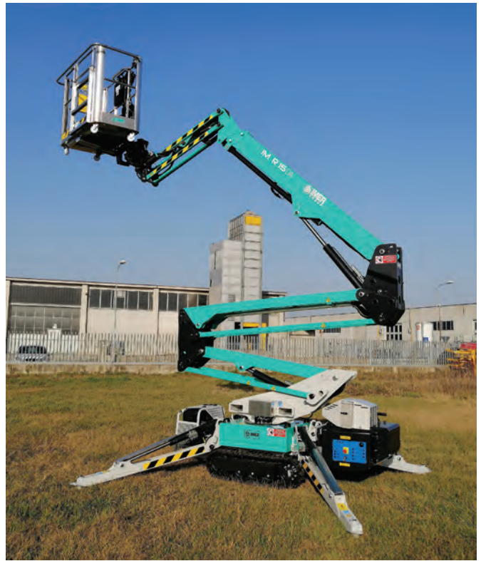
ALL IMAGES: Imer IM R 15 DA tracked platform features a working height of 15.10 m and double articulated boom with active jib. The machine has a maximum payload capacity of 230 kg.
