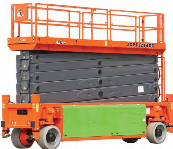
ABOVE AND LEFT: Dingli JCPT3214DC electric rough-terrain scissor lift offers a maximum working height of 32 m. Its maximum platform height is 30 m.
