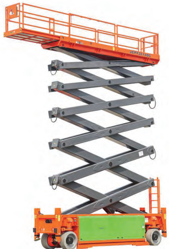
ABOVE AND LEFT: Dingli JCPT3214DC electric rough-terrain scissor lift offers a maximum working height of 32 m. Its maximum platform height is 30 m.
